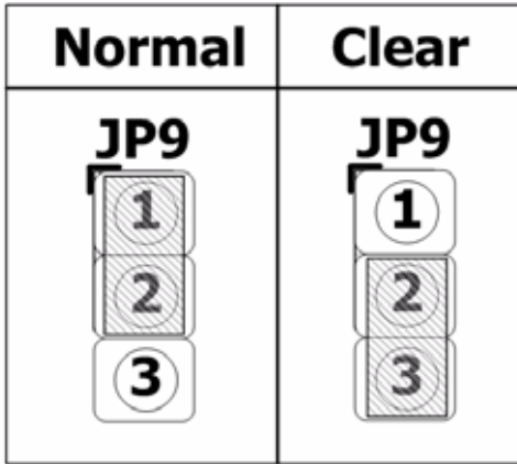
Figure 2-17: JP9 (Clear CMOS) Settings
