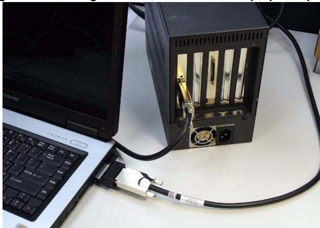
Figure 2-4: Cabling 3 M Extension Cable to Laptop Computer
