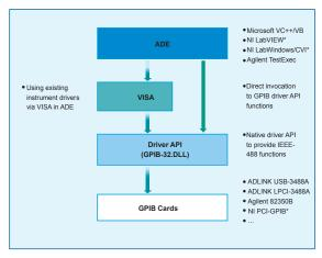
work with your applications in both ways. Its GPIB-32.DLL provides binary compatibility with the popular NI-488.2\* driver software. The USB-3488A and LPCI-3488A also provide VISA library support that can be used with most common instrument drivers written by instrument vendors. Regardless if you are using VC++, VB, Delphi, LabVIEW\*, or any other T&M ADE, ADLINK GPIB interface cards are the most cost-effective GPIB solutions compatible with all your applications.
