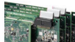
SSI bus cable for multiple cards synchronization
